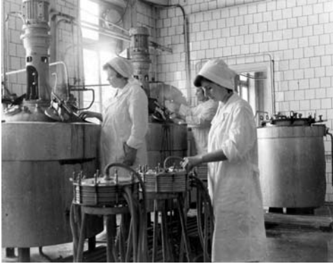
Figure 5.8 Workers pump finished phage solution through the round sterile filters at the Tbilisi institute in the 1970s
